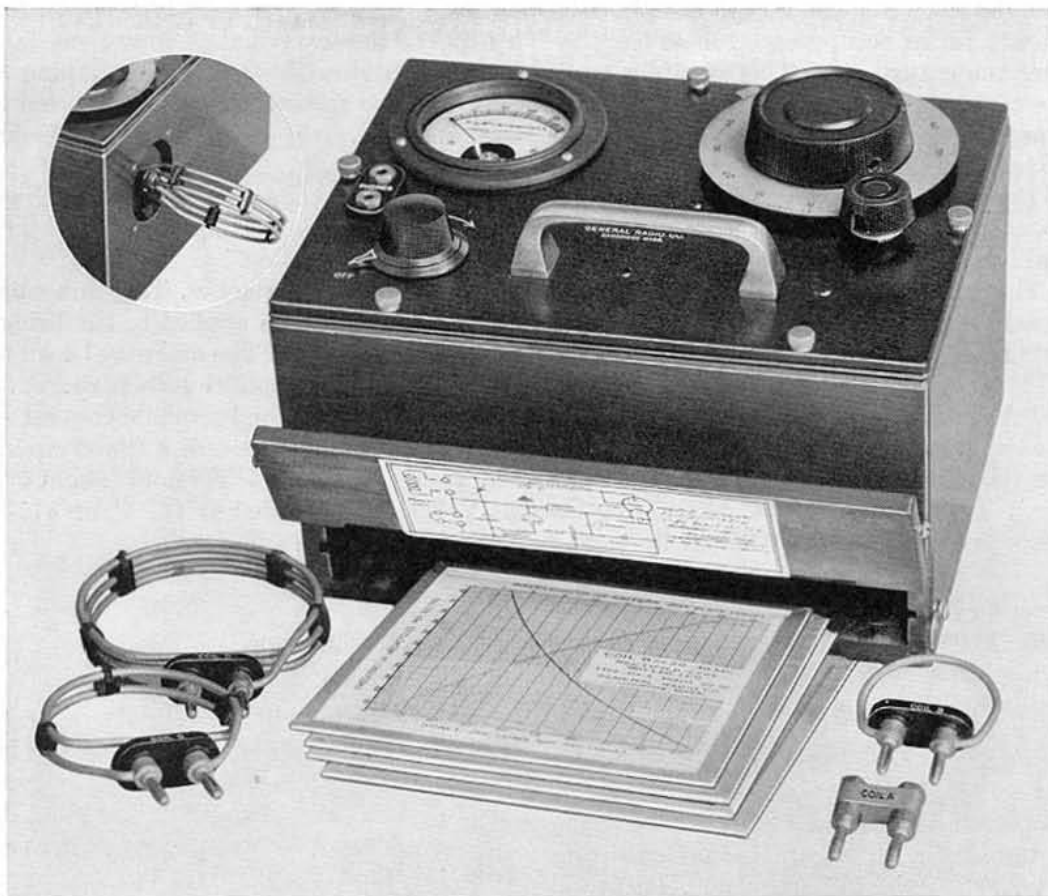
A TYPE 419-A Rectifier-Type Wavemeter with the four inductors and their individual calibration charts. The insert shows the method of plugging in an inductor
