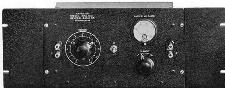
The TYPE 514-AR Amplifier for mounting in a standard 19-inch relay rack
